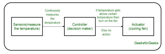
The control system acts upon an environment through the actuator. It requires a source of energy and a control signal. When it receives a control signal, it converts the source of energy to a mechanical operation. On this basis, on which form of energy it uses, it has different types given below.
